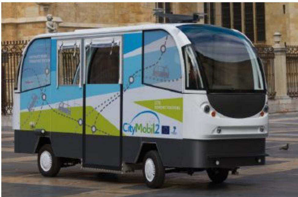
The CityMobil 2 prototype is a fully electric and driverless minibus that can carry up to 10 passengers and reach a top speed of 40 Km per hour, seen here in the city of León, Spain
