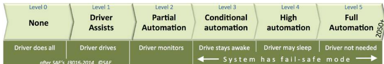
Figure 1: The SAE standard description for automated vehicle levels.
