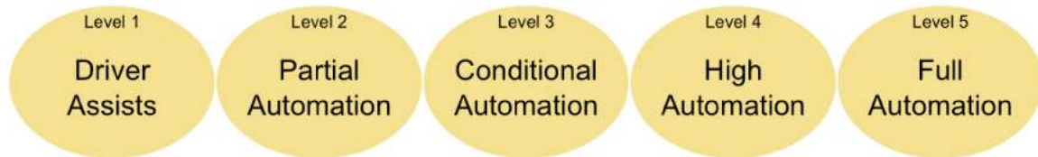
Figure 2: Stages of Vehicle Automation as set out by the Society of Automotive Engineers 4
