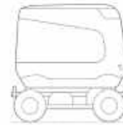
Starship Robot 10 kg 6 km/h
